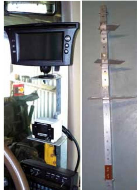
**Mounting tree holds 3 or more monitors in one location, and is easy to see and operate from tractor seat.**
