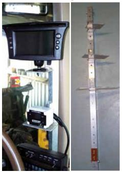
Mounting tree holds 3 or more monitors in one location, and is easy to see and operate from tractor seat.
