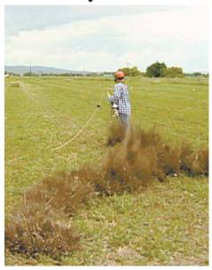
A mixture of oxygen and propane are injected underground and then ignited by the Rodenator to kill underground pests. You can see videos, photos and more information at the company's website: www.rodenator.com.
