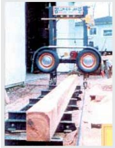
Reeks first sawmill, the Lum-BR-Jak, was built in 1994 from miscellaneous parts for less than \$100.
