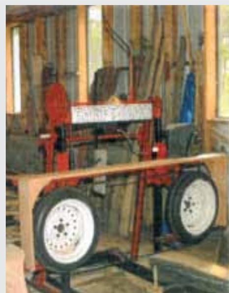
In 2010 Reeks designed his latest new sawmill, the Thriftwood. It's powered by a single phase 220-V motor. No fumes so it can be used inside.
