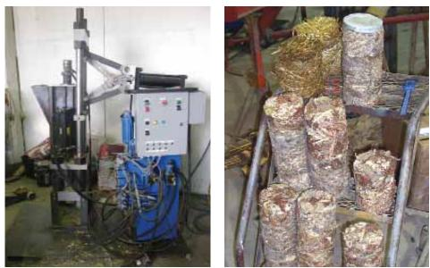
Large-scale pelletizer presses switchgrass or corn stalks into 6-in. dia. "pellets".
