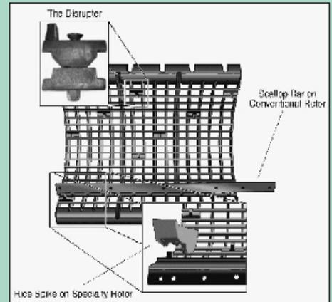
Disrupter improves crop flow and reduces grain loss in crops that are tough to thresh.
