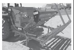
Bale shredder attaches to a 3-pt. hitch or quick-taches to a front-end loader.
