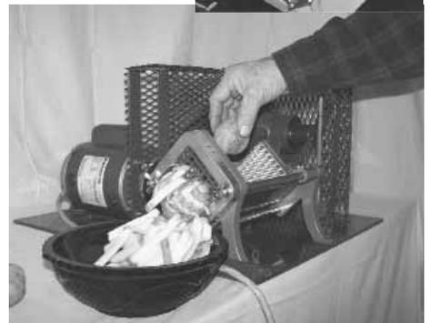
To make French fries, operator drops in one potato at a time and uses a foot pedal to activate the potato pusher.
