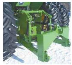
Mandako also makes Cat. III hitches, such as this one mounted on a Deere 4630.
