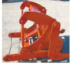
Cat. IV hitch allows 4-WD articulated tractors to lift big equipment, such as 24-row planters and 50-ft. wide field cultivators.
