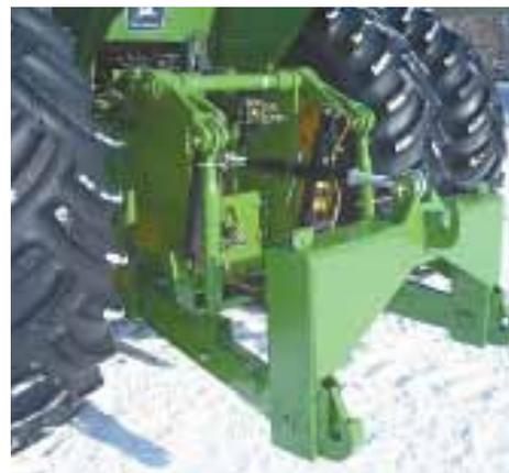
Mandako also makes Cat. III hitches, such as this one mounted on a Deere 4630.
