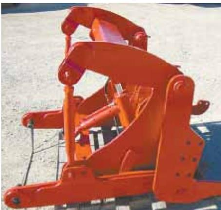
Cat. IV hitch allows 4-WD articulated tractors to lift big equipment, such as 24-row planters and 50-ft. wide field cultivators.
