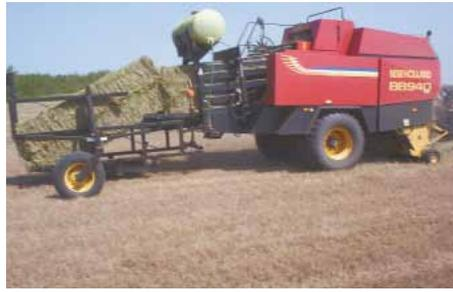
**Caster wheel-mounted bale stacker is designed to always trail in line with baler's bale chute.**
