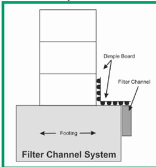
The system works well in most soils, the only exception being fine sand. If you are installing it in fine sand, or you're concerned about your soil plugging the system, just apply a minimum of 2 in. of BB shot rock (1/8 to 1/4-in.) or concrete sand around the mesh drain to prevent it from plugging. It's a lot less work than the amount of rock necessary to install a 3-in. drain tile system.
