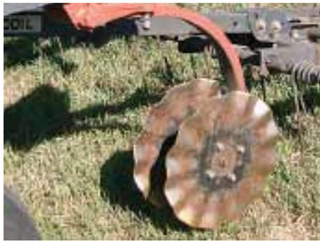
Coupler kit includes 18-in. 13-wave boron "earthenharden" coupler blades, left. Kit, right, is now fitted with 4 bearings to make it even more heavy-duty. Works in wheat stubble and corn stalks. Cuts up trash so you can plant days earlier.
