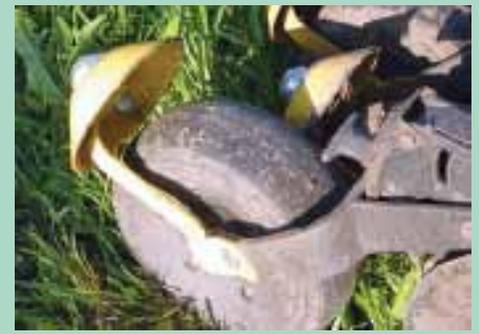
Rotating "cup scrapers" bolt onto air seeder's packer wheel mounting arm at about a 45 degree angle. Scraper is offset 1 in. from center of packer wheel.
