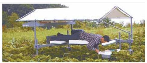
Battery-powered picking cart comes with a vinyl canopy that protects both the crop and the operator from sun or rain.
