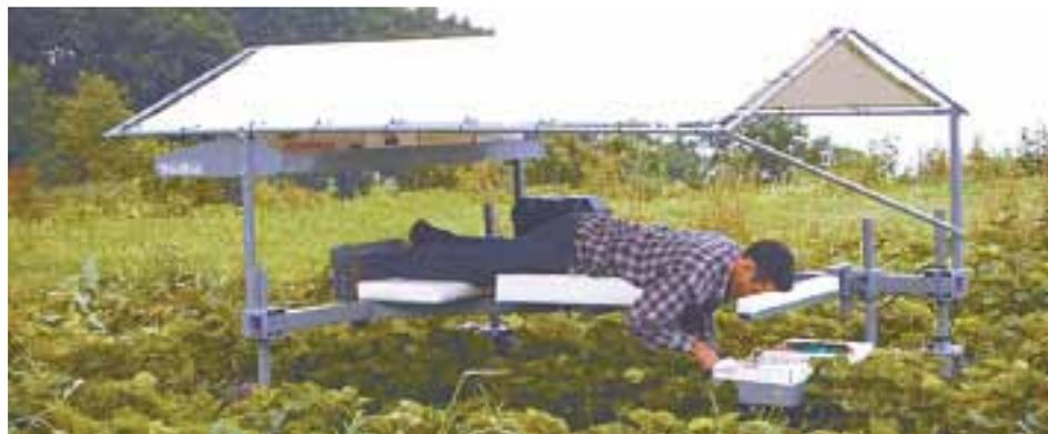
**Battery-powered picking cart comes with a vinyl canopy that protects both the crop and the operator from sun or rain.**
