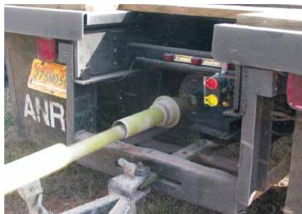
to run a bagger machine. He and his son-in-law run a self-propelled forage harvester for their custom harvesting business. A lot of time was wasted arranging to get the tractor to run the bagger. Adding a pto to a truck makes the bagging operation self-sufficient.
