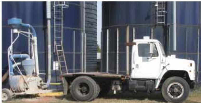
This 200 hp plus truck is attached to a grain-vac. Notice the pto gear box and the live hydraulics (below).
