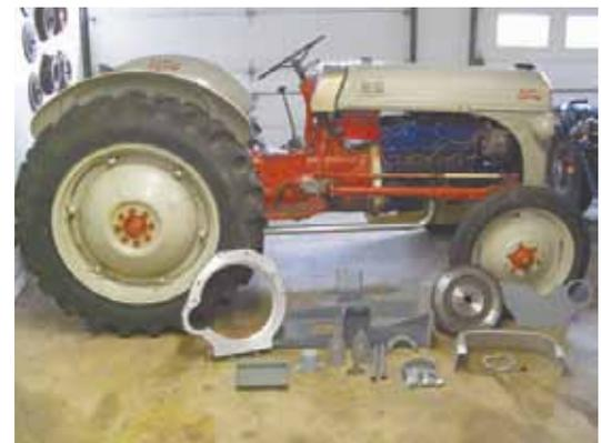
**Photo shows parts included in overhead valve conversion kit for N-Series Fords.**
