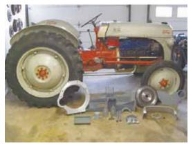
Photo shows parts included in overhead valve conversion kit for N-Series Fords.
