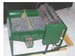
When the treadle is pumped up and down, connecting rods turn the reel and shake the screen.
