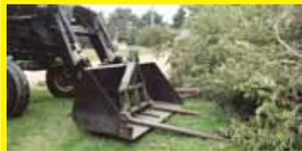
There seem to be a lot of fancy ways to mount forks on a loader bucket. We simply chain our 3-pt. forks into the bucket to give the rig a bigger bite for loading tree limbs and brush. Works great. **(Rex Gogerty, Hubbard, Iowa)**
