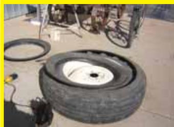
We needed turf tires for our tractor but could not justify them. So we bought some old, bald truck tires that were 1/2 size bigger than the tractor tires. We cut 2 to 2 1/2 in. off the inside of each tire sidewall and slid them onto the tractor tires, then reinflated. Works great and we no longer leave tracks from lugged tires when spraying weeds. **(Andy, Delta, Colo.)**
