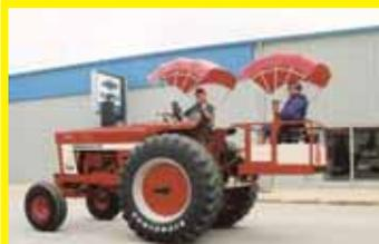
tractor for parades, tractorcades, or crop tours. It attaches to the tractor's 3-pt. hitch and has a sun shade, easy step, and an entry door with an air-ride seat. It's made from heavy-duty steel with white plywood trim to match the tractor. **(Dennis Neubauer, 31491 Co. Hwy. S27, Garden City, Iowa 50102, ph 515 893-2320)**
