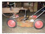
Push lawn mower has pipe bolted on top that fits inside trailer's coupler.
