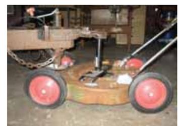
Push lawn mower has pipe bolted on top that fits inside trailer's coupler.
