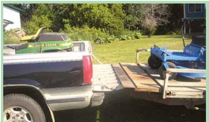
Hinged, latch-operated panel on front of trailer folds forward onto pickup's tailgate.
