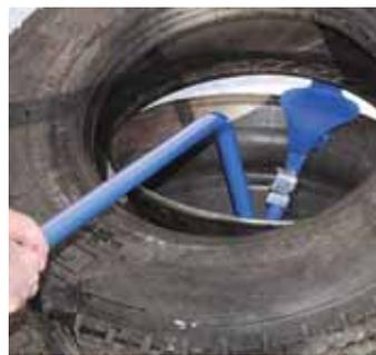
It works because of the patented shape of the tool's head, and the leverage that you get from the handle.
