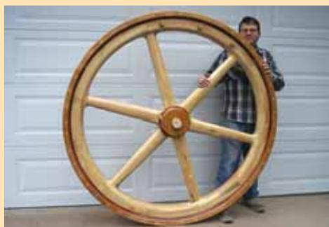
Gary Martin makes models for castings, ranging from miniature parts for antique tractor collectors to man-sized steam engine flywheels.
