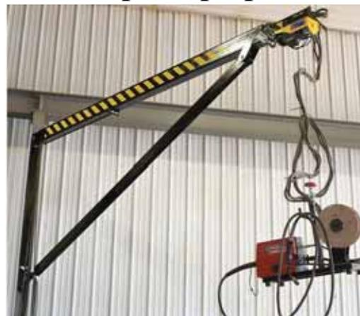
Welder hangs from cable on wall-mounted boom that can swivel up to 180 degrees.
