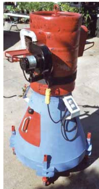
To reshape hard steel, Brian Johnson uses heating and forging furnaces that he built himself using a beer keg and a propane tank.
