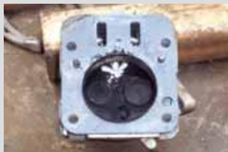
like a bird's foot where I used a rotary end mill file on a milling machine to make the grooves in the engine head.
