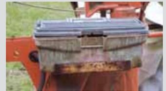
**Chad Travis, Drasco, Ark.:** "I mounted a standard, off-the-shelf 14-in. long toolbox on the hitch of my Kuhn 3-pt. mounted, 8-ft. rotary hay mower. I used angle iron and flat steel to make a mounting bracket for the toolbox that welds to the hitch frame. The toolbox bolts to the bracket.
