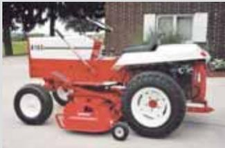
"The tractor was completely disassembled and every part was sand blasted and painted before reassembly. The forward and reverse clutches were replaced as well as the bushings and bearings in the front axle and the rear axle hubs. The 16 hp Briggs & Stratton engine was beyond repair. I ended up installing a 20 hp Honda V-twin engine purchased from Northern Tool, which required only minimal modifications. The new engine runs smooth, and the extra
