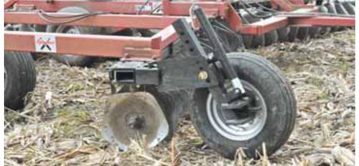
Falk installed a set of the blades on his Case IH 496 28-ft. disk and calls it a Rolling Spader.
