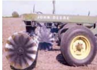
He straightened out the gangs and put straight/wavy coulters on them, both front and back.
