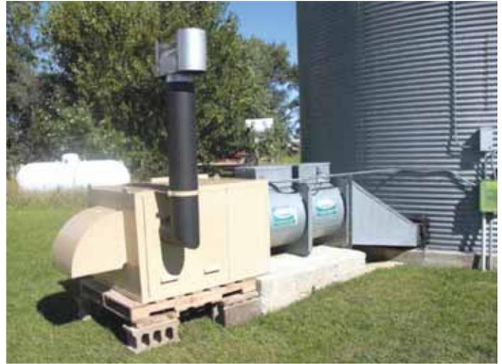
**Desert Air Crop Dryer uses a heat exchanger between the burner and fan to enable it to dry grain with drier, cleaner air than conventional dryers.**
