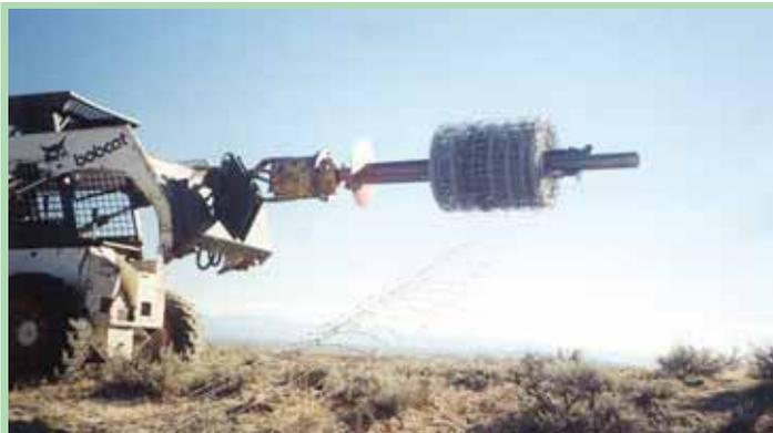
Faced with the job of removing 72 miles of woven wire, Randy Sloan invented this wire roller that attaches to a hydraulic post hole auger on a skid loader.
