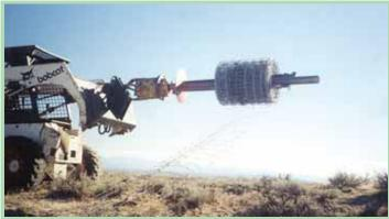
Faced with the job of removing 72 miles of woven wire, Randy Sloan invented this wire roller that attaches to a hydraulic post hole auger on a skid loader.
