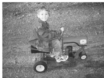
Made to look like a Deere, mini tractor is powered by the 2-stroke motor and built-in clutch off an Echo weedeater.
