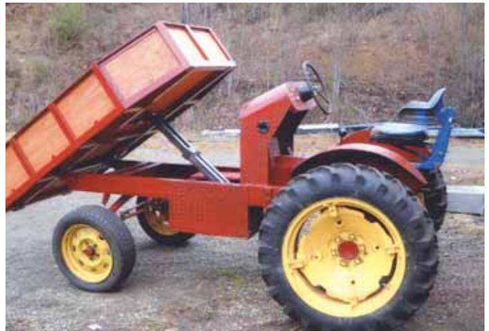
Dave Benoit converted this 1948 Massey Harris Pony tractor to electric power, adding a plywood dump box on front.
