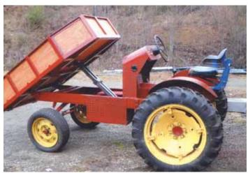
Dave Benoit converted this 1948 Massey Harris Pony tractor to electric power, adding a plywood dump box on front.
