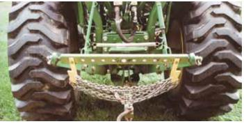
An old tractor drawbar mounts horizontally between tractor's lower lift arms. Logging chain is wrapped around a pair of U-shaped metal brackets on drawbar
