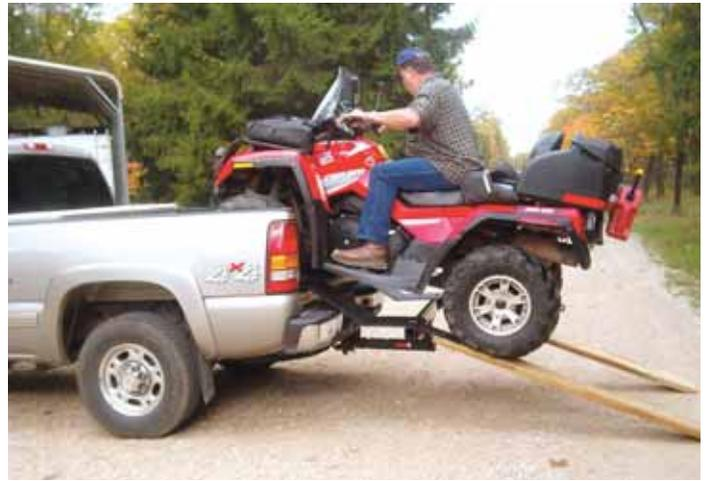
ATV's rear wheels are held securely in wheel pans molded into the wheel ramps.
