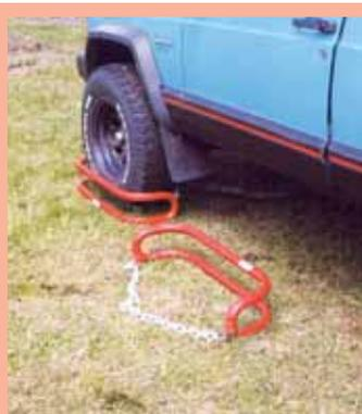
"Tire lock" is made from 1 1/4-in. dia. pipe bent and welded together to wrap around front and back sides of tire. A chain welded to one end of unit wraps around frame.
