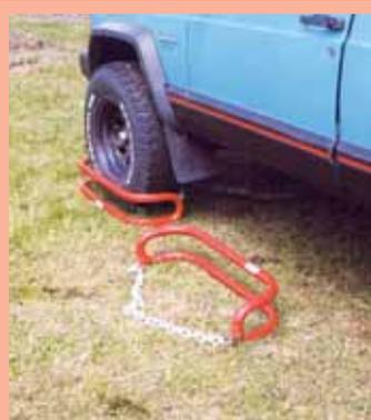
"Tire lock" is made from 1 1/4-in. dia. pipe bent and welded together to wrap around front and back sides of tire. A chain welded to one end of unit wraps around frame.
