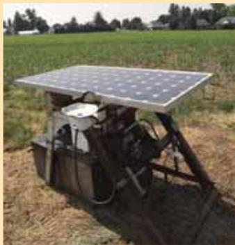
Winch and its solar panel mount to a 2,000-lb. block of concrete that Nolt moves as needed.
