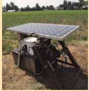
Winch and its solar panel mount to a 2.000-lb. block of concrete that Nolt moves as needed.
