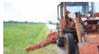
**Mowing steep road ditches isn't a problem for Jerry Scott with this sidewinder mower that he made from a conventional 72-in. belly mount. His rig has 3 ft. of up and down travel and can mow 30-degree angle ditches.**
