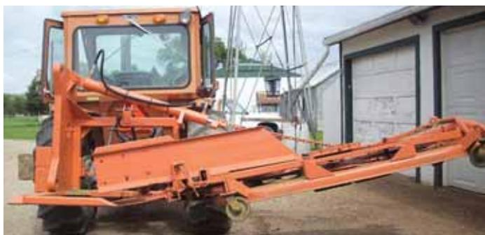
**Six old tractor weights mounted to the left side of the 3-pt. frame counter balance the 72-in. mower when it's in a raised position.**
