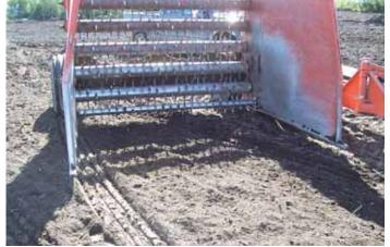
Root piler has 6 horizontal rollers spaced 4 in. apart, with 3 rows of teeth that spiral from the outside to the middle.
