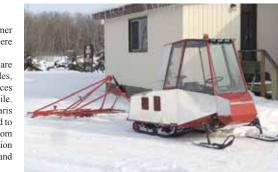
Home-built snowmobile trail groomer has a heated cab, allowing Mysko to work without a jacket in temperatures down to 40 degrees below zero.
