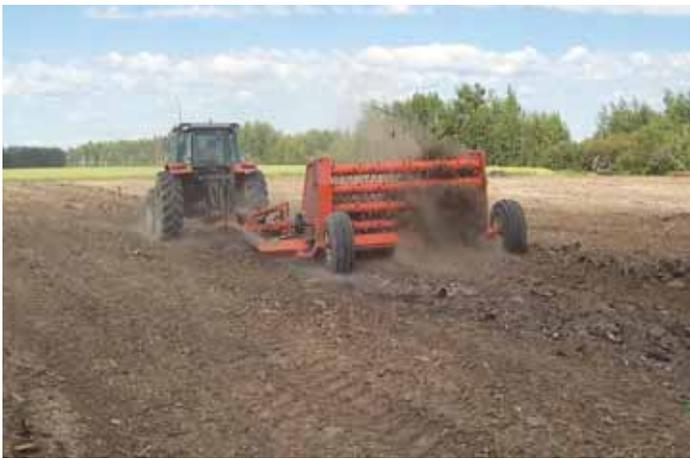
Home-built “root piler” moves everything from 2-in. dia. roots to 12-in. dia. logs up to 8 ft. long. It makes an 8-ft. wide swath.
