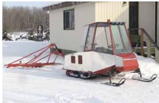
Home-built snowmobile trail groomer has a heated cab, allowing Mysko to work without a jacket in temperatures down to 40 degrees below zero.
