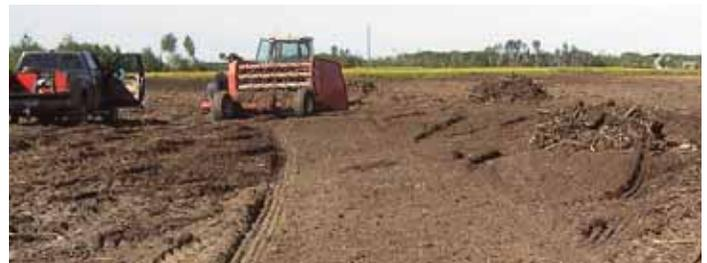
Operator drives slowly as piler rolls roots ahead of it until pile reaches 3 to 4 ft. high and can’t roll any more. Then he backs up, drives around pile and continues.
