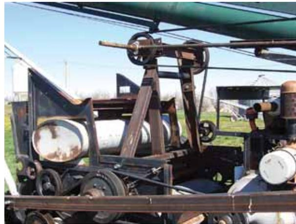
Auger is driven by double groove pulleys from the combine, and its separator clutch stops and starts the auger.
