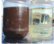
Jack Benner operates a fuel-cleaning service that comes to farms. Photo shows fuel before and after it has been cleaned.
