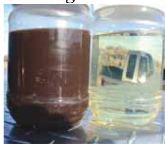
Jack Benner operates a fuel-cleaning service that comes to farms. Photo shows fuel before and after it has been cleaned.
