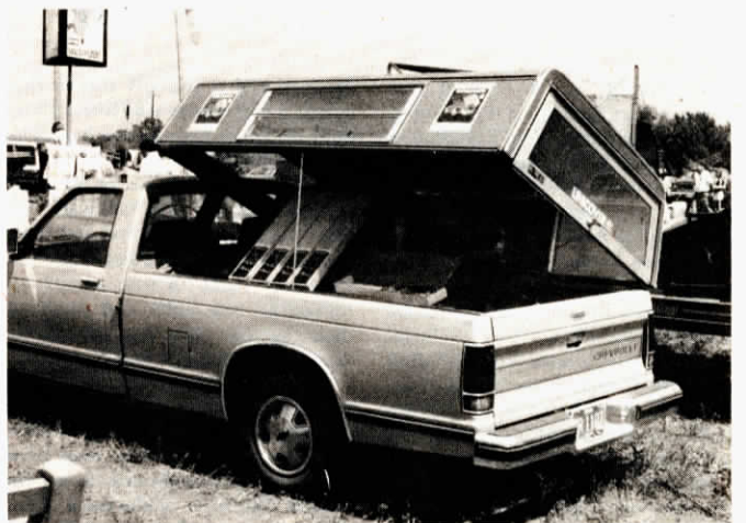
Three hinges along one side of the topper are all it takes to convert it for "easy open" access.
