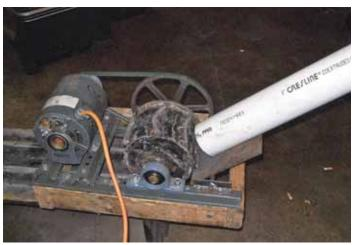
Bruce Olp installed powered can crusher in the basement of his bar and restaurant. Pvc tube runs through hole in floor and down to crusher.
