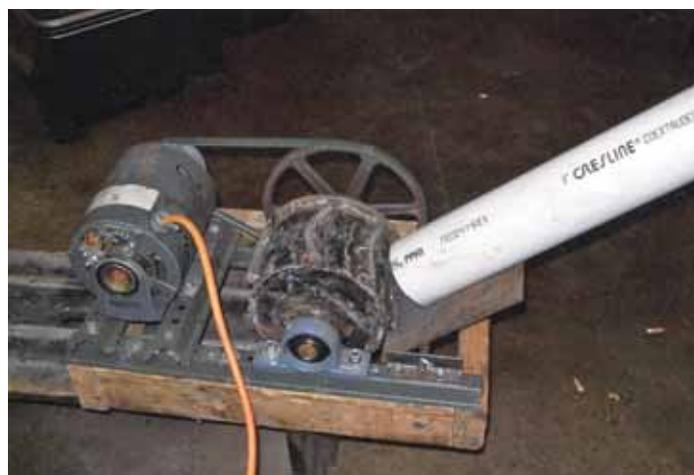
Bruce Olp installed powered can crusher in the basement of his bar and restaurant. Pvc tube runs through hole in floor and down to crusher.
