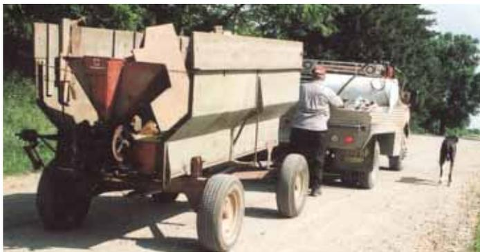
To keep dust down on the gravel road in front of his home, this farmer near Zeoring, Iowa, has been spreading calcium chloride with an old endgate seeder.
